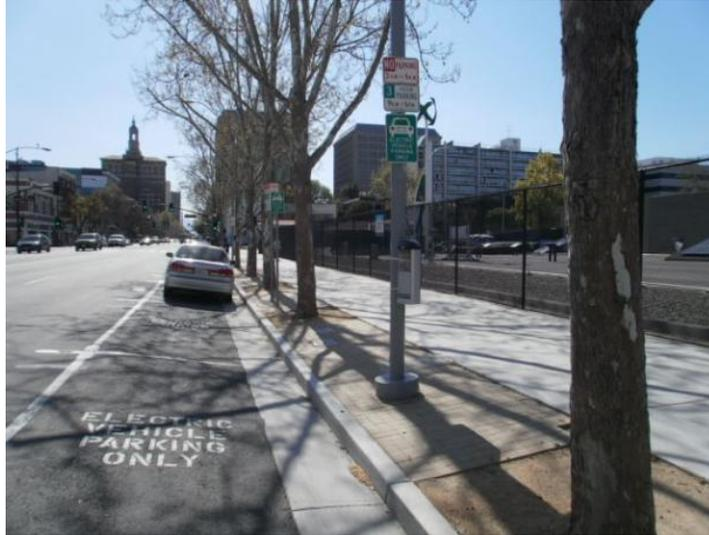
Figure 25. On-Street E.V.C.S. (charger & signs on streetlight pole)
