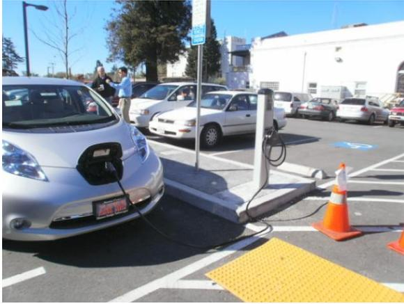
Figure 7. Accessible E.V.C.S. in parallel space on opposite side of two accessible parking spaces. Ecology Action Parking Lot, Santa Cruz, Ca.
