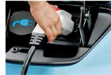
The J1772 connector will be the standard charging plug for all new electric vehicles.
